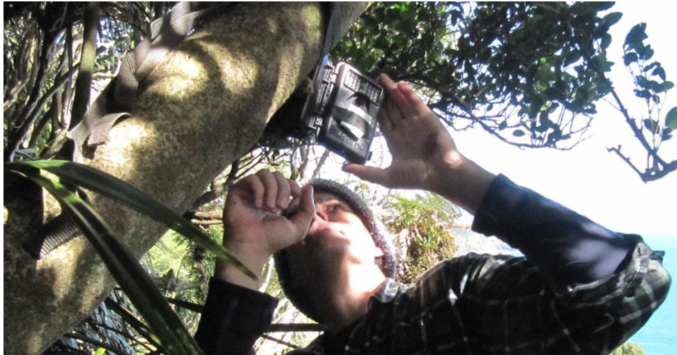
Thomas Mattern changing the batteries and memory card in one of the motion activated cameras. Jackson Head, September 2014.
